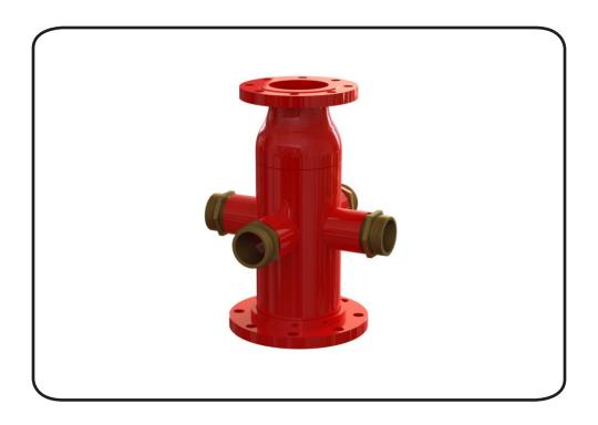
Hydrant Base for monitors 6" (152 mm) flanged inlet with 4" (102mm) flanged outlet for mounting monitor. Base has four 2-1/2" (64mm) outlets for extending water lines in high risk areas. Can be either flat or raised face flange. Carbon steel body with red powder coating.
